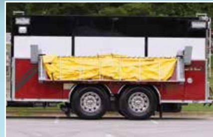
▼ Powered Drop Tank Storage
